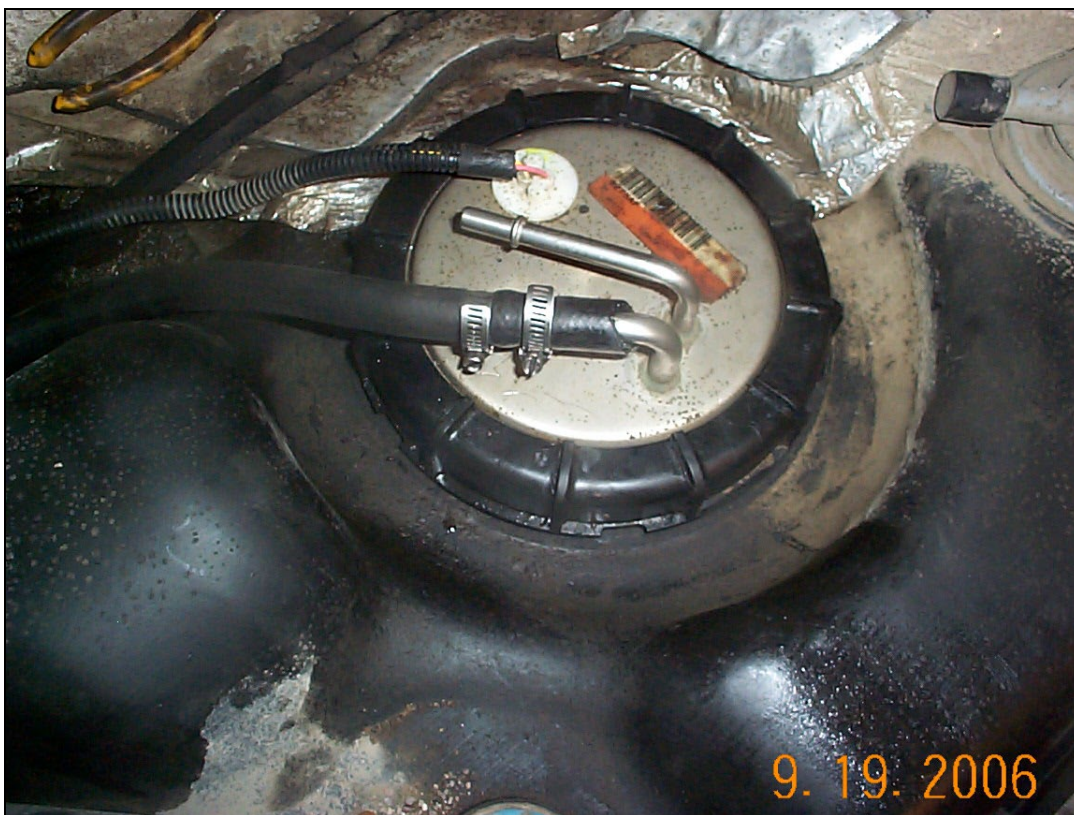
Figure 15 – New Fuel Line Double Clamped on Pickup Tube (Excursion Shown)
