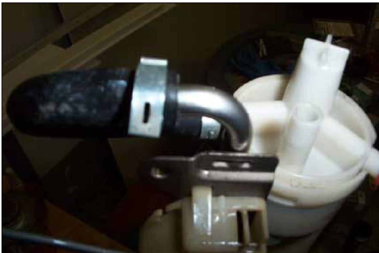
Figure 4 - Cutting The Factory Return Line Hose Clamp
