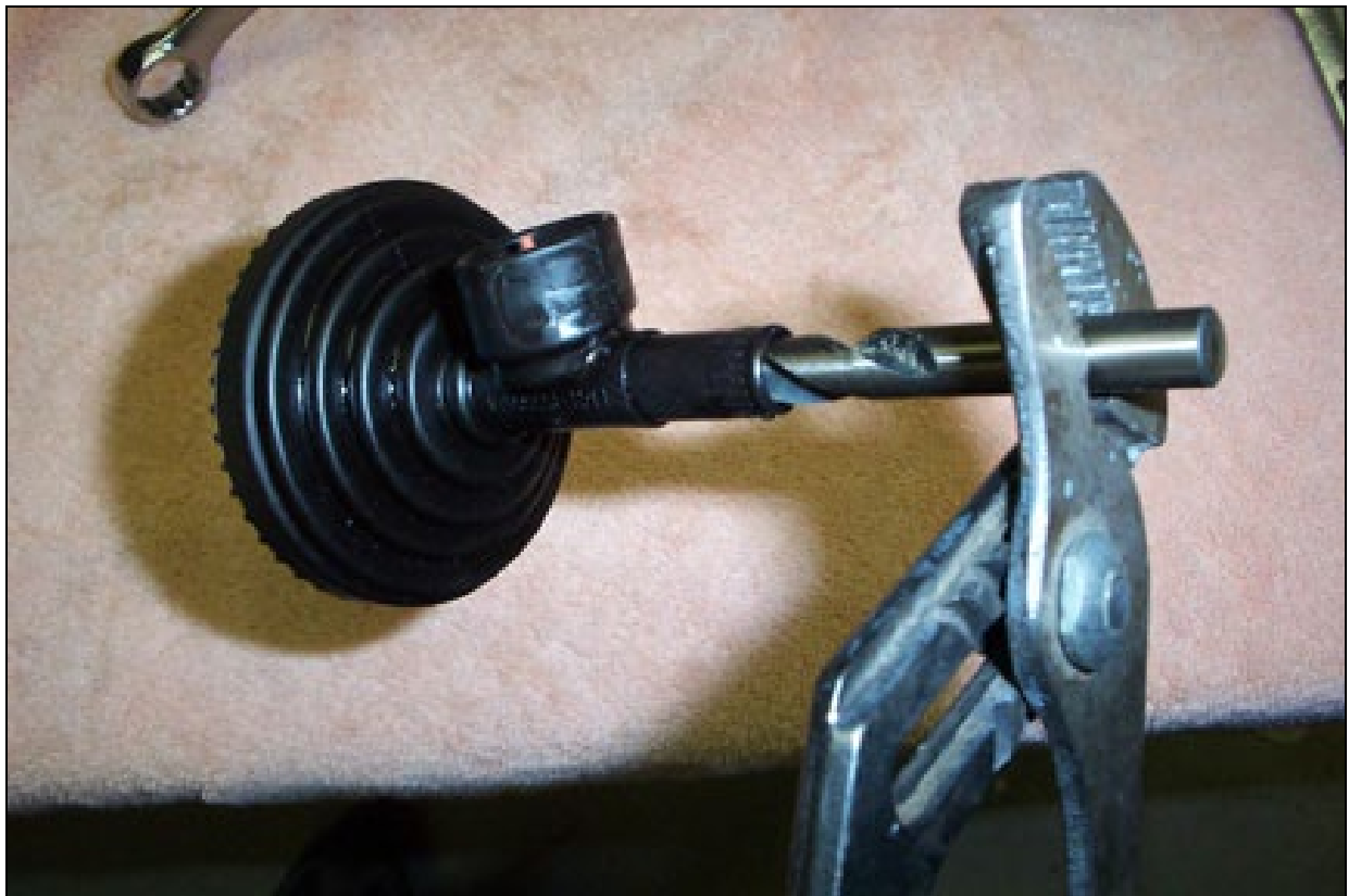
Figure 8 – Clearancing Pickup Strainer for Pickup Tube
