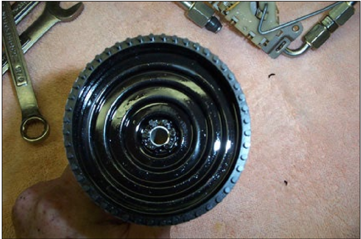
Figure 9 – Pickup Tube Installed in Strainer
