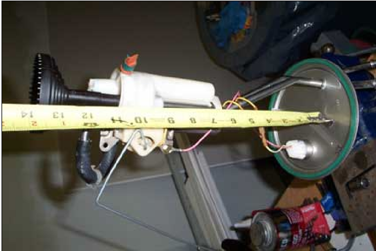
Figure 3 - Measuring The Factory Strainer Depth
