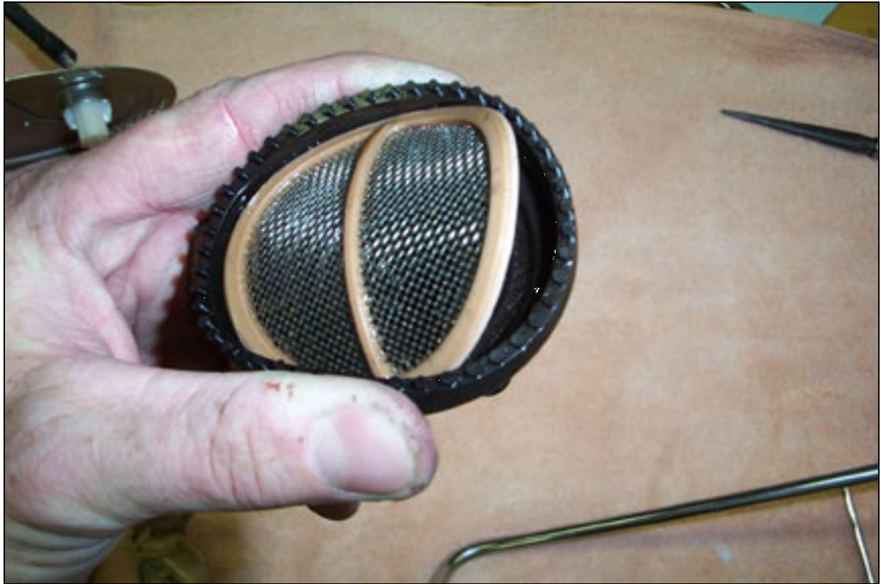
Figure 7 – Removing Filter Screen From Strainer
