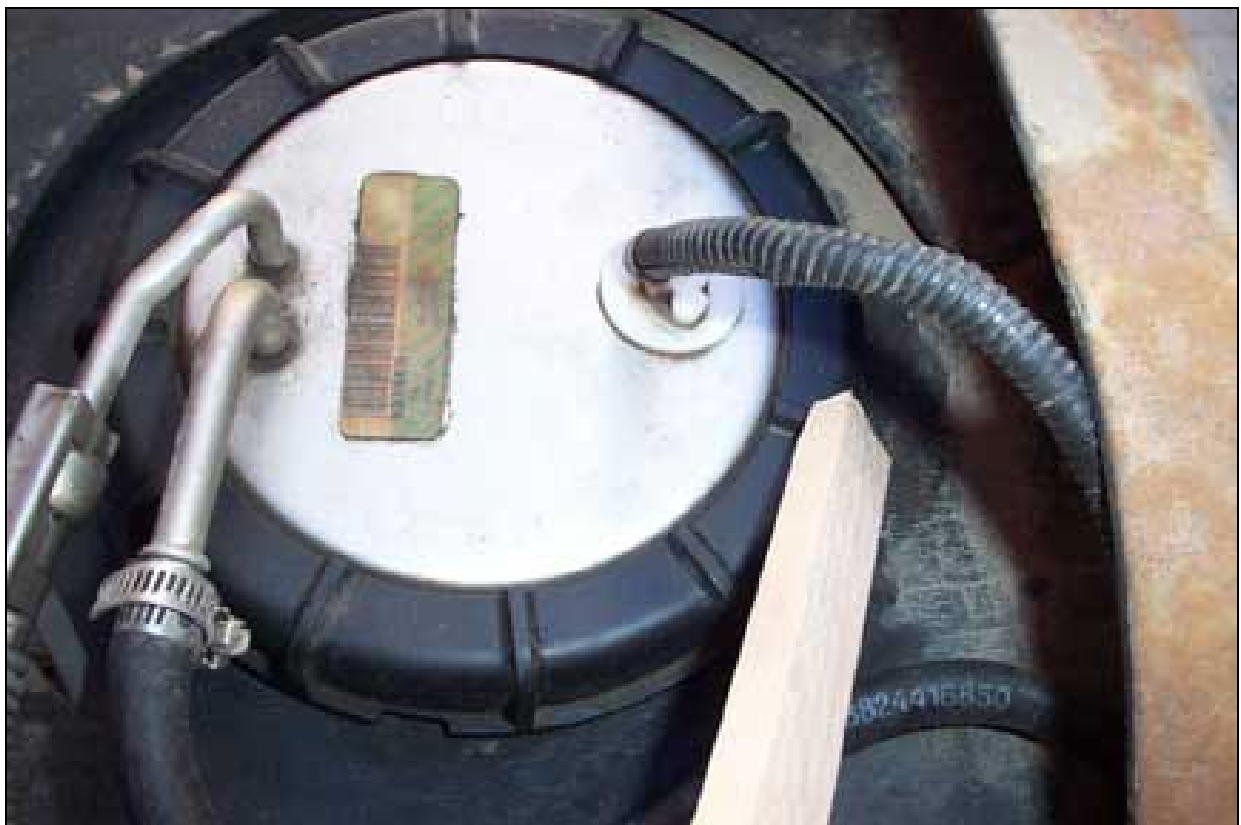
Figure 2 - Removing The Sending Unit Retention Ring
