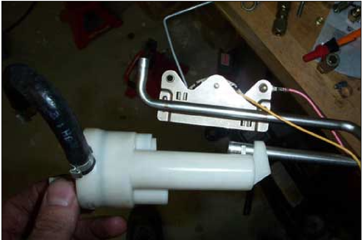
Figure 5 - Removing The Mixing Chamber
